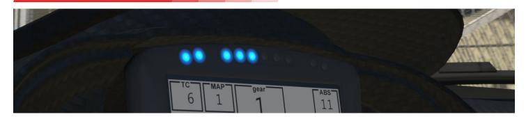
When the pit limiter is active the first 5 shift light LED's will illuminate in blue.
