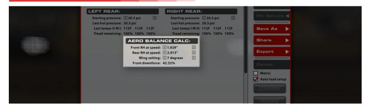
The Aero Calculator is a tool provided to aid in understanding the shift in aerodynamic balance associated with adjustment of the rear wing setting and front and rear ride heights. It is important to note that the values for front and rear ride height displayed here DO NOT result in any mechanical changes to the car itself, however, changes to the rear wing angle here WILL be applied to the car. This calculator is a reference tool ONLY.
